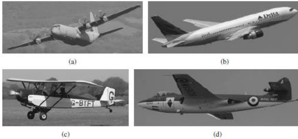
Figure 3.7. Four aircraft with different wing vertical positions: (a) Lockheed Martin C-130J Hercules (high wing); (b) Boeing 767 (low wing); (c) Pietenpol Air Camper-2 (parasol wing); (d) Hawker Sea Hawk (mid-wing)
