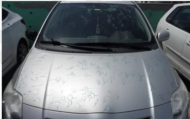
Figure 1. Damage caused by hailstones to a vehicle Source: https://www.cnnturk.com/
