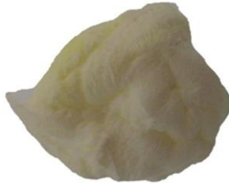
Figure 3. An image of a water-based artificial hailstone containing 12% PVA material after melting
