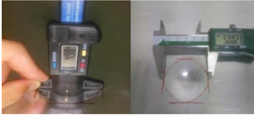
Figure 16. Measurement of dent depth and diameter in 0.3 mm steel panels
