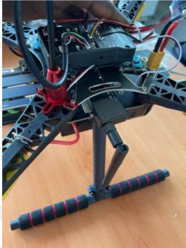
Figure 6.9. GPS module stand attached to the frame.
