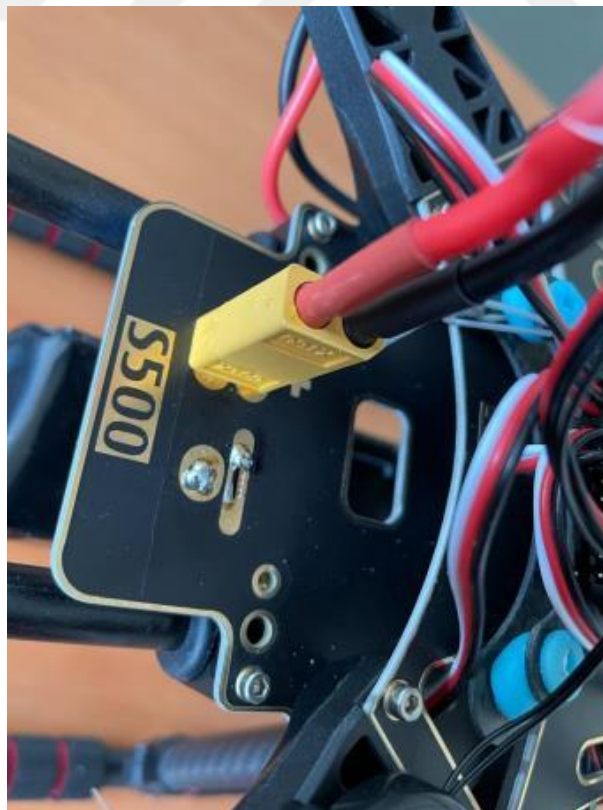
Figure 6.10. Soldering of the power module XT60 connector.
