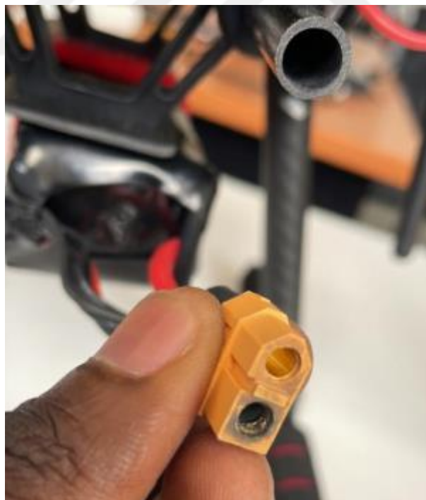
Figure 5.1. Burned power module.
