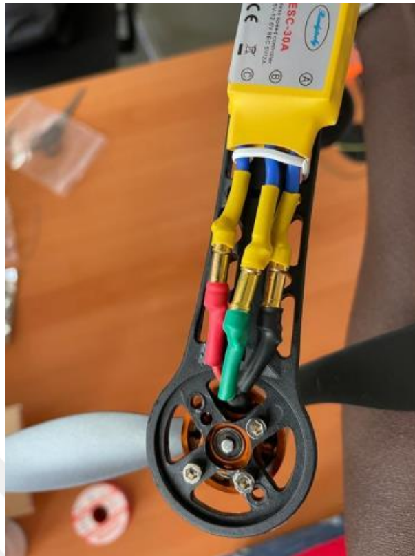
Figure 6.7. ESC to Motor connection using Banana connectors.
