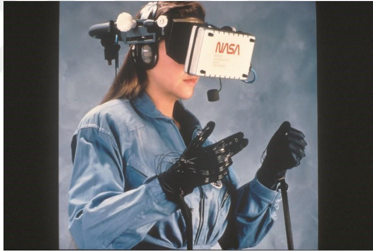
Resim 1.5. The Virtual Interface Environment Workstation (VIEW)
