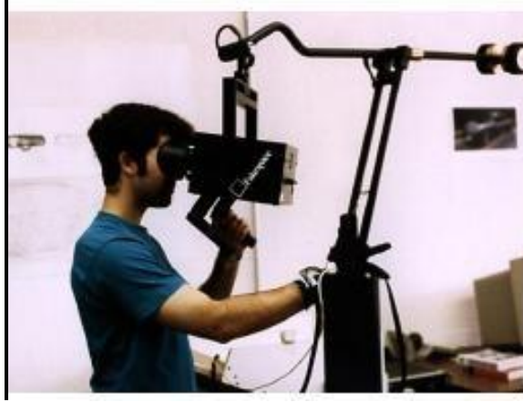
Resim 1.7. BOOM (Binocular Omni-Orientation Monitor)
