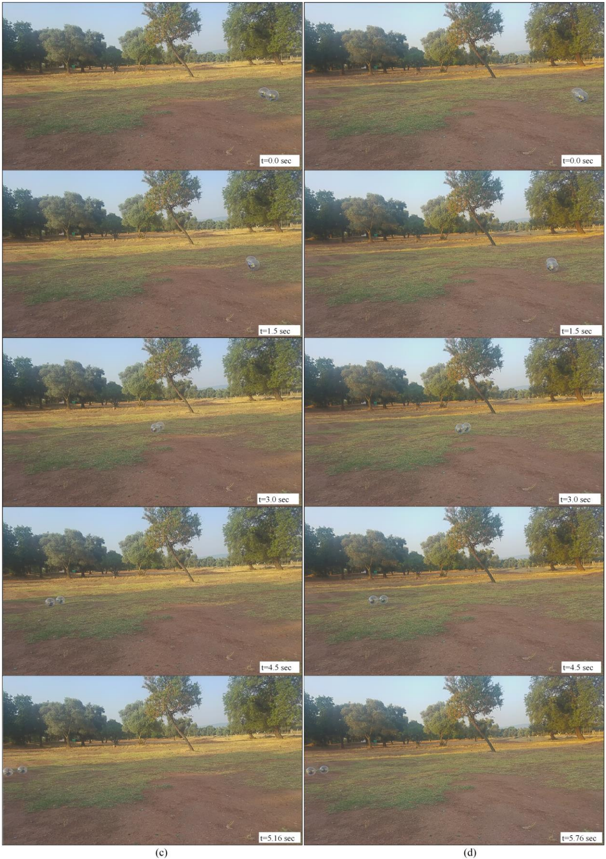
Figure 62: Video snapshots of second random road experiments (side) (c) two identical coupled spherical robots which with torsional soft spring connection (d) two identical coupled spherical robots which with torsional stiff spring connection
