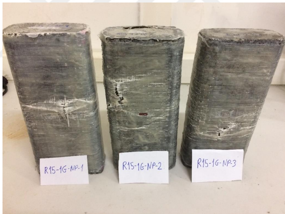
Picture 4.3. Failure modes of R15-1G-NP specimens
