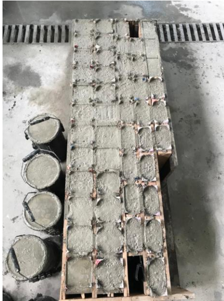
Picture 3.4. The formwork after casting the concrete
