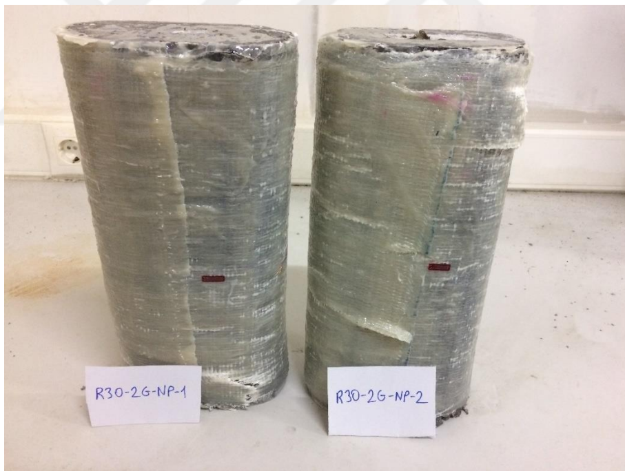
Picture 4.9. Failure modes of R30-2G-NP specimens
