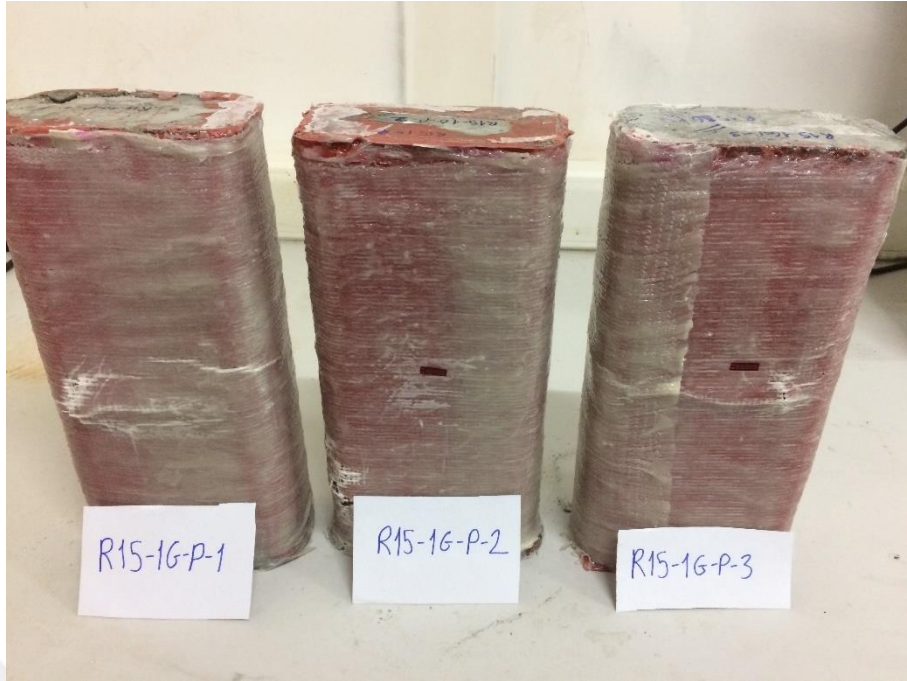
Picture 4.4. Failure modes of R15-1G-P specimens
