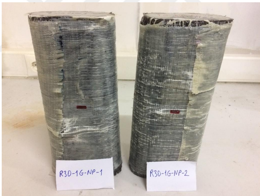
Picture 4.7. Failure modes of R30-1G-NP specimens
