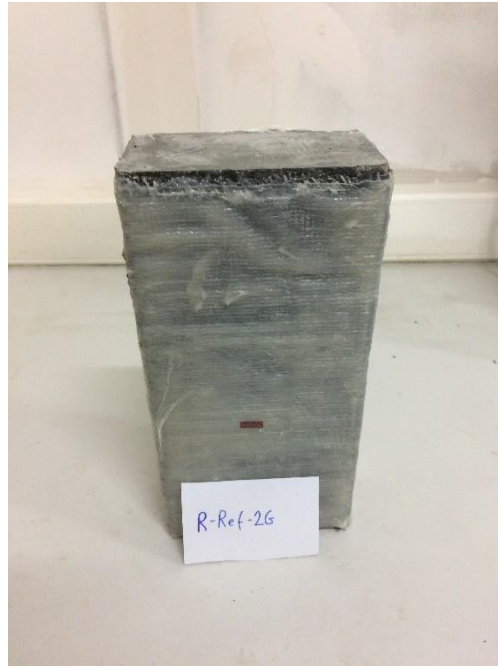
Picture 4.2. The failure mode of the specimen with sharp edges confined with two layers of GFRP
