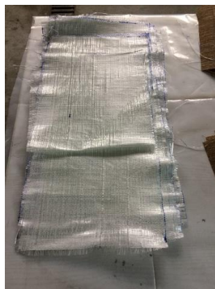
Picture 3.8. GFRP sheets prepared with the determined dimensions
