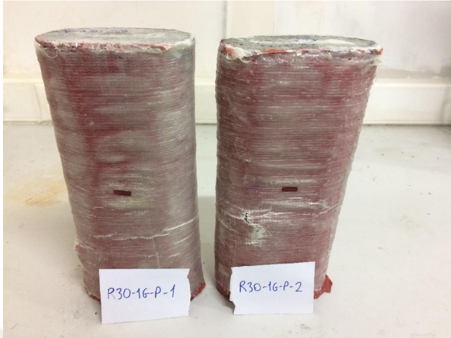
Picture 4.8. Failure modes of R30-1G-P specimens
