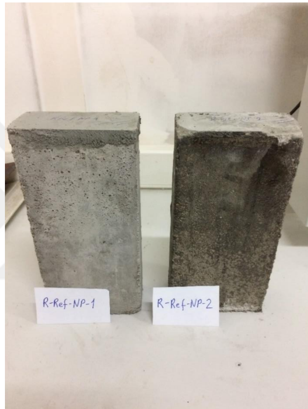
Picture 4.1. Failure modes of unconfined specimens
