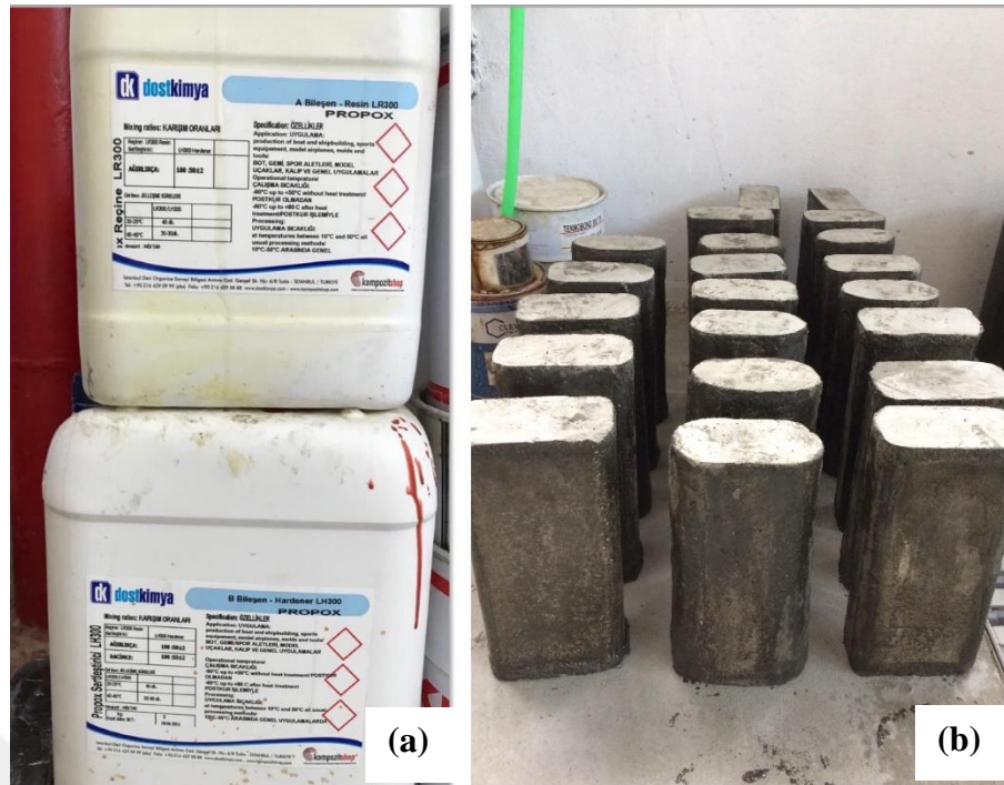
Picture 3.6. (a) The components of the primer (b) The specimens after application of primer
