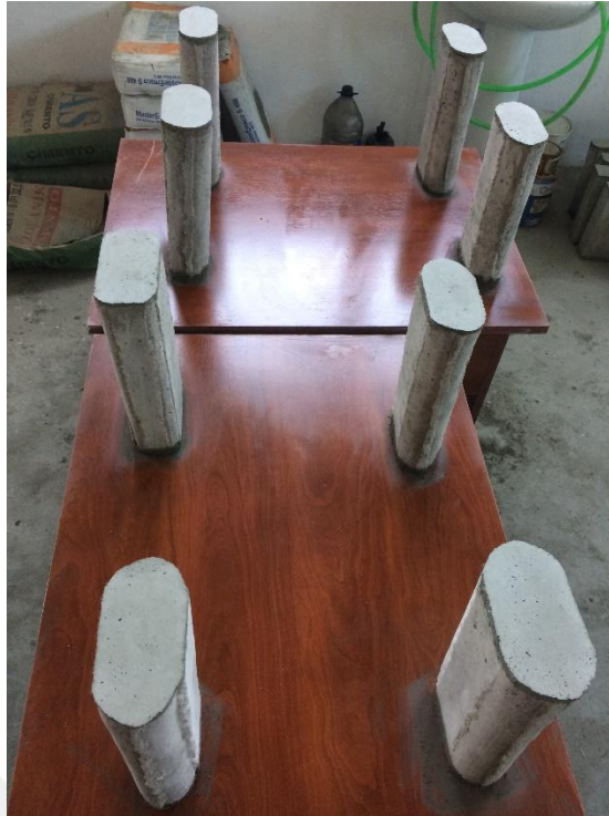
Picture 3.5. The specimens after capping the ends
