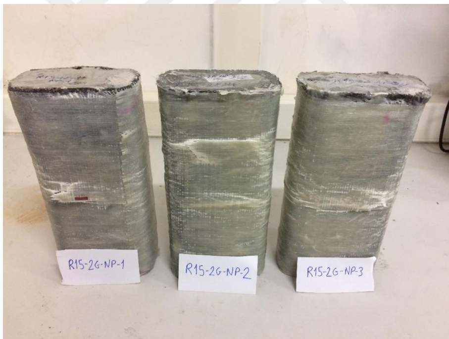
Picture 4.5. Failure modes of R15-2G-NP specimens
