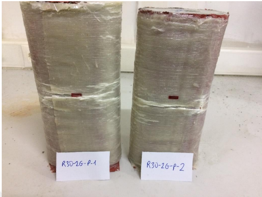
Picture 4.10. Failure modes of R30-2G-P specimens
