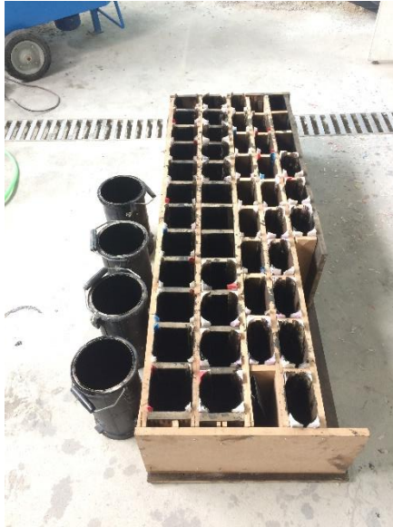
Picture 3.2. The formwork after oil applied into inner surfaces
