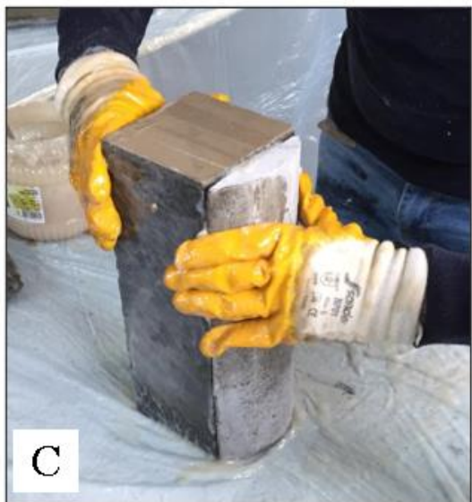
Picture 3.11. Steps of implementing the shape modification technique for the unrounded-corners of the core, a) top view for the core and the concrete segments, b) applying the epoxy on the surface of the specimen and the concrete segment, c) attaching the specimens on the surface of the core, and d) the final shape of the specimen.
