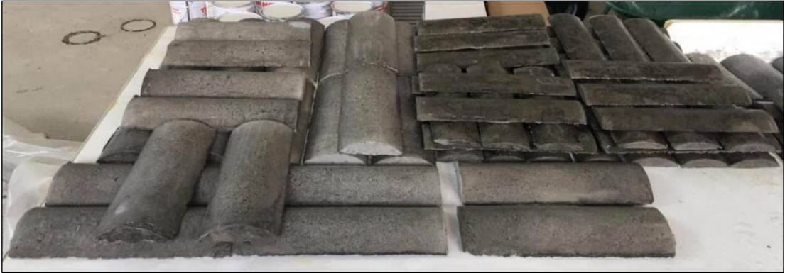
Picture 3.5. Concrete segments after taking them out of the water pool
