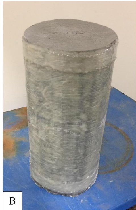
Picture 3.16. CRCF group, a) applying the epoxy primer, and b) wrapping the GFRP sheet
