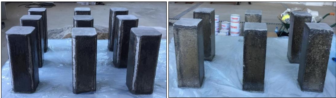
Picture 3.8. Concrete specimens after applying the primer on the flat surfaces
