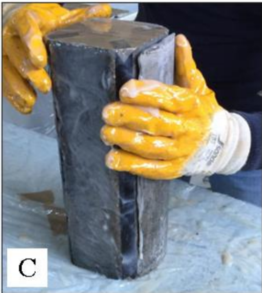
Picture 3.10. Steps of implementing the shape modification technique for the rounded-corners of the core, a) top view for the core and the concrete segments, b) applying the epoxy on the surface of the specimen and the concrete segment, c) attaching the specimens on the surface of the core, and d) the final shape of the specimen.
