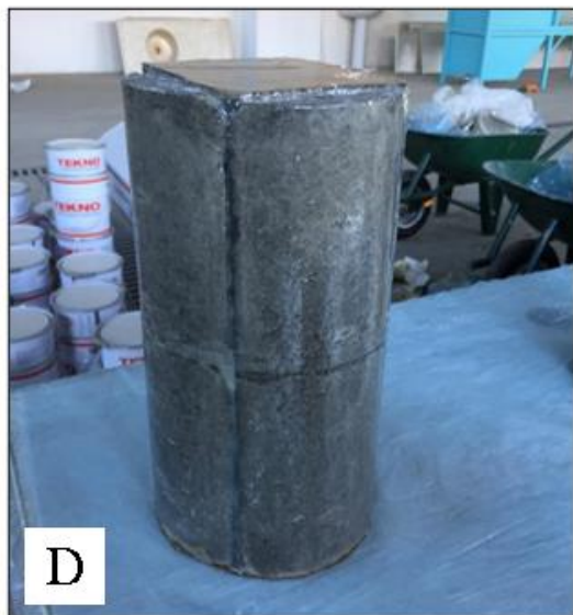
Picture 3.11. Steps of implementing the shape modification technique for the unrounded-corners of the core, a) top view for the core and the concrete segments, b) applying the epoxy on the surface of the specimen and the concrete segment, c) attaching the specimens on the surface of the core, and d) the final shape of the specimen.
