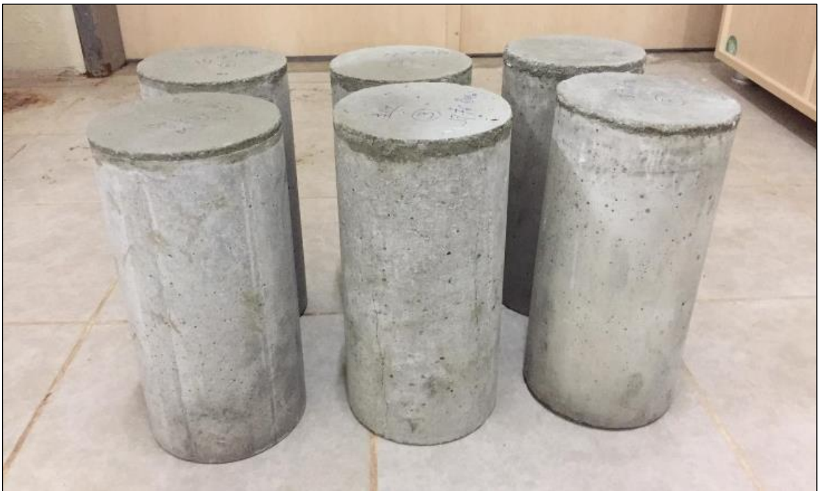
Picture 3.19. Concrete cylinders to test the compressive strength after 28 days.
