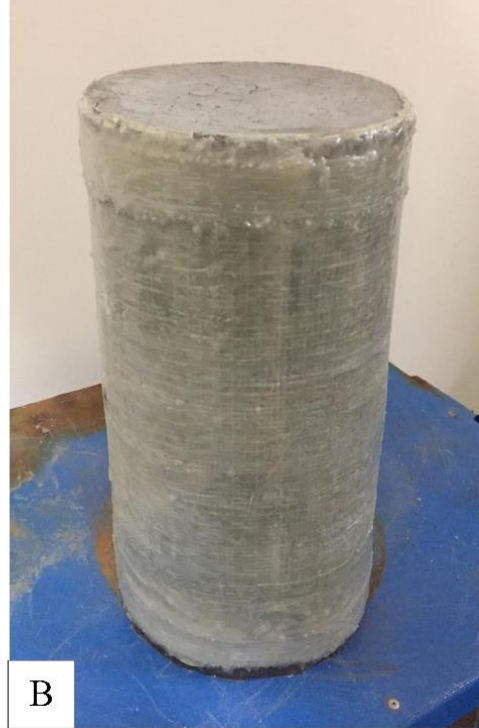
Picture 3.15. CCF group, a) applying the epoxy primer, and b) wrapping the GFRP sheet.
