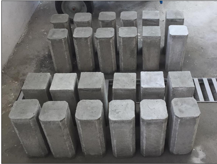
Picture 3.7. Concrete specimens after capping the ends
