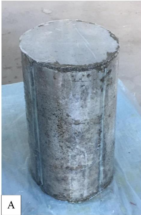
Picture 3.15. CCF group, a) applying the epoxy primer, and b) wrapping the GFRP sheet.
