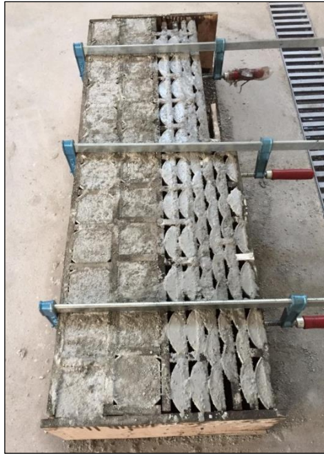
Picture 3.2. The formwork after casting the concrete
