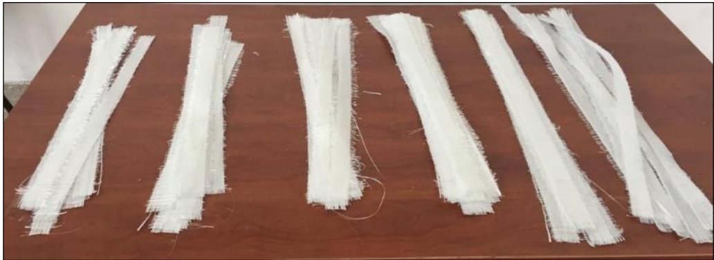
Picture 3.12. GFRP sheets and rings after the cutting process.
