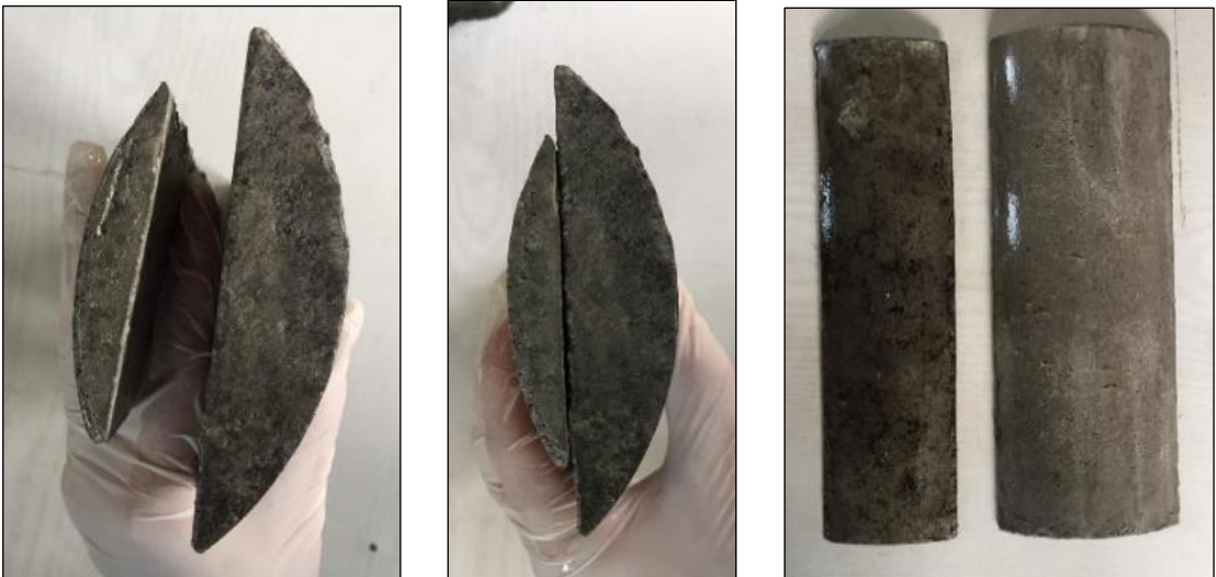
Picture 3.6. Size difference between the concrete segment of the proposed shape modification method and the previous shape modification method
