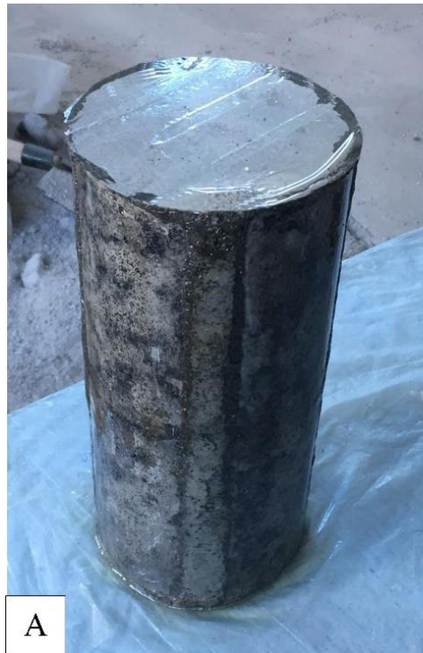
Picture 3.16. CRCF group, a) applying the epoxy primer, and b) wrapping the GFRP sheet
