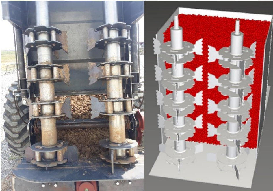
Figure 3.7. Compost Particle Injection in Solid Spreader
