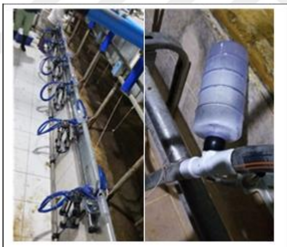
Figure 3.1. Removable individual milk yield apparatus from private animal breeders of Aydın.
