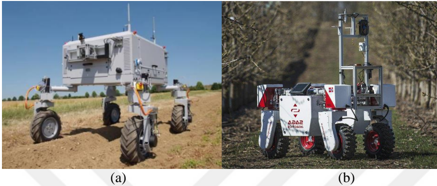
(a) (b) Figure 2.17 Mobile Robots Used In Agriculture: a) Bonirob Developed By BOSCH Deepfield-Robotics (Bosh, 2019), b) Thorvald was Designed By SAGA ROBOTICS (Saga Robotics, 2019).
