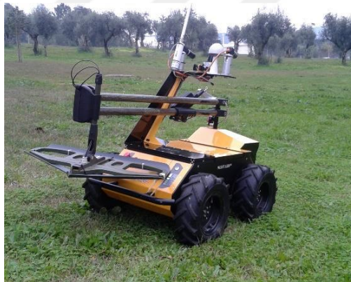
Figure 2.18 Husky with Mechanisms That Make Him Prepared To Detect Mines (Cabrita Et Al., 2015).
