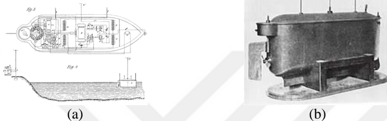
Figure 2.1 The Robot Boat (A) Patent Drawing (B) Structure (Rosheim, 1994)
