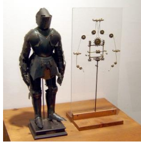
Figure 2.30. Armored knight and its inner working mechanism
