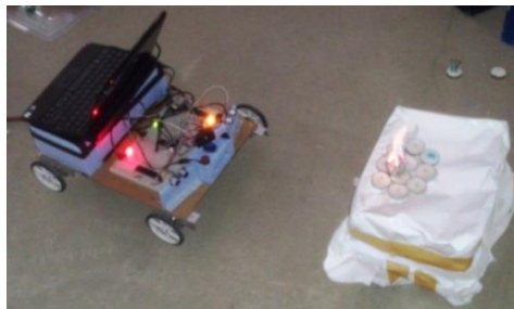
Figure 4.36. Fire detection based on distance test
