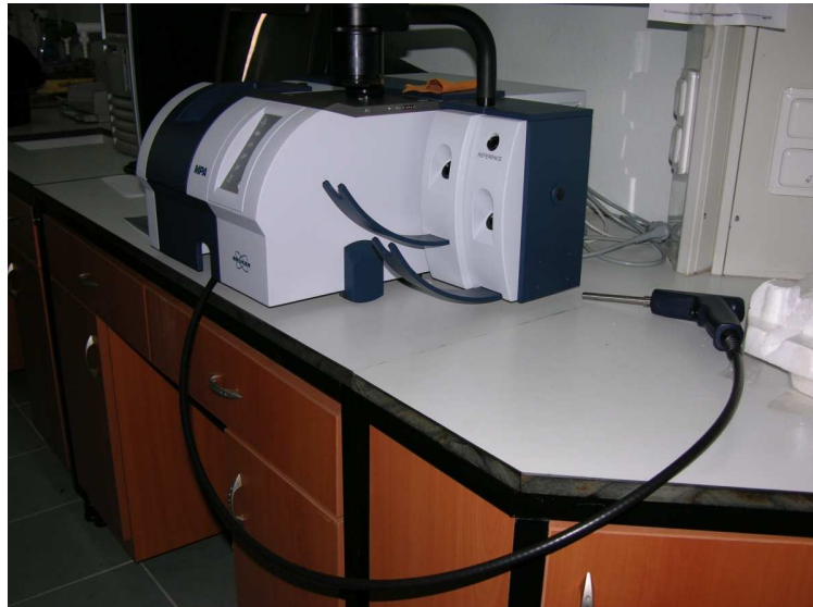
Fig. 2. FT-NIR spectrometer used in the study
