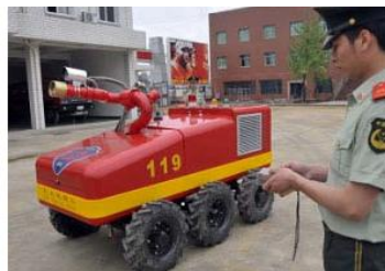
Figure 2.51. JMX-LT50 firefighting robot
