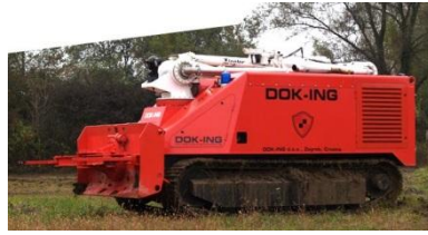
Figure 2.50. MVF-5 firefighting robot
