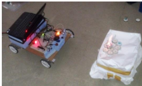
Figure 4.36. Fire detection based on distance test
