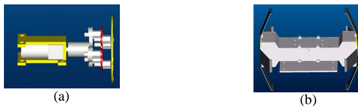
Figure 2.61. Impact resistance mechanisms of Kim's robot (a) leaf spring (b) side bolster
