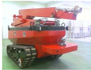
Figure 2.55. MyBOT 2000 firefighting robot
