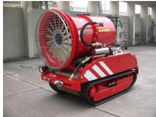
Figure 2.46. LUF60 firefighting robot
