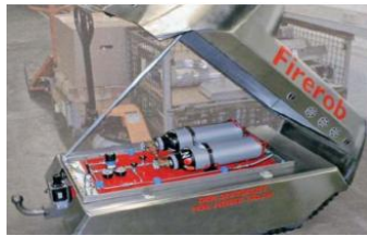
Figure 2.47. FIREROB firefighting service robot
