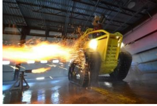
Figure 2.54. Thermite T2 firefighting robot
