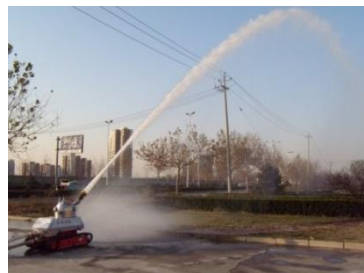
Figure 2.49. Firemote firefighting robot
