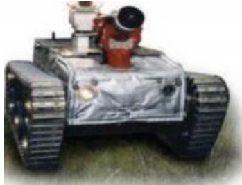
Figure 2.48. FFR-1 firefighting robot
