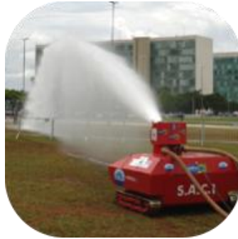
Figure 2.52. SACI 2.0 firefighting robot
