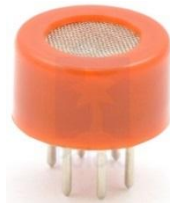
Figure 3.14. MQ-9 carbon monoxide and flammable gas sensor
