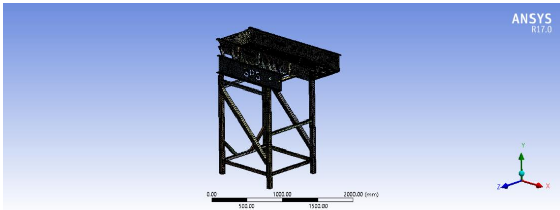
Figure 5.10. Mesh for Vibratory conveyor
