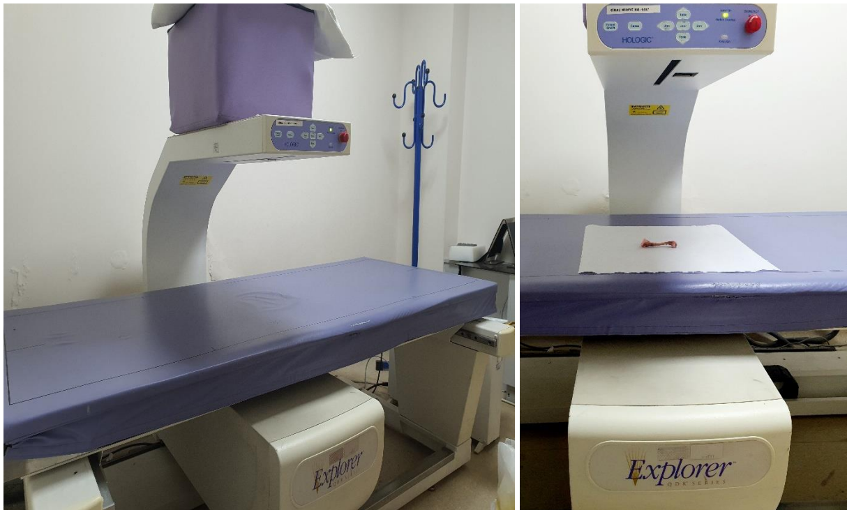
Figure 20. DEXA apparatus with tibia sample ready for scanning.
