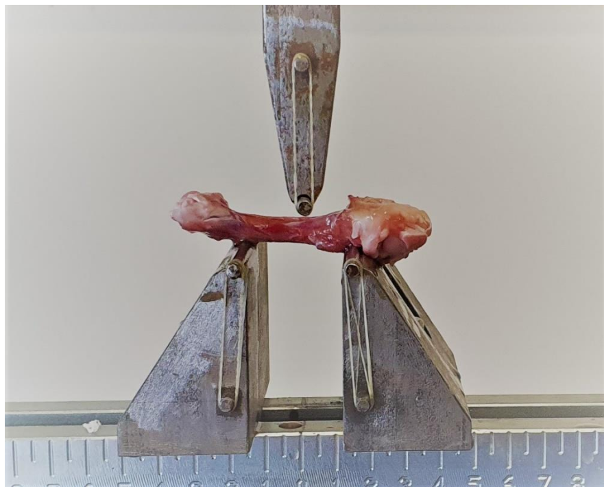
Figure 26. Three-point bending test of humerus.
