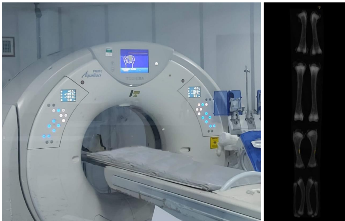
Figure 4. Represents the CT apparatus and position of all the bones of one chicken in a scanogram (right and left), arranged on CT table for scanning.
