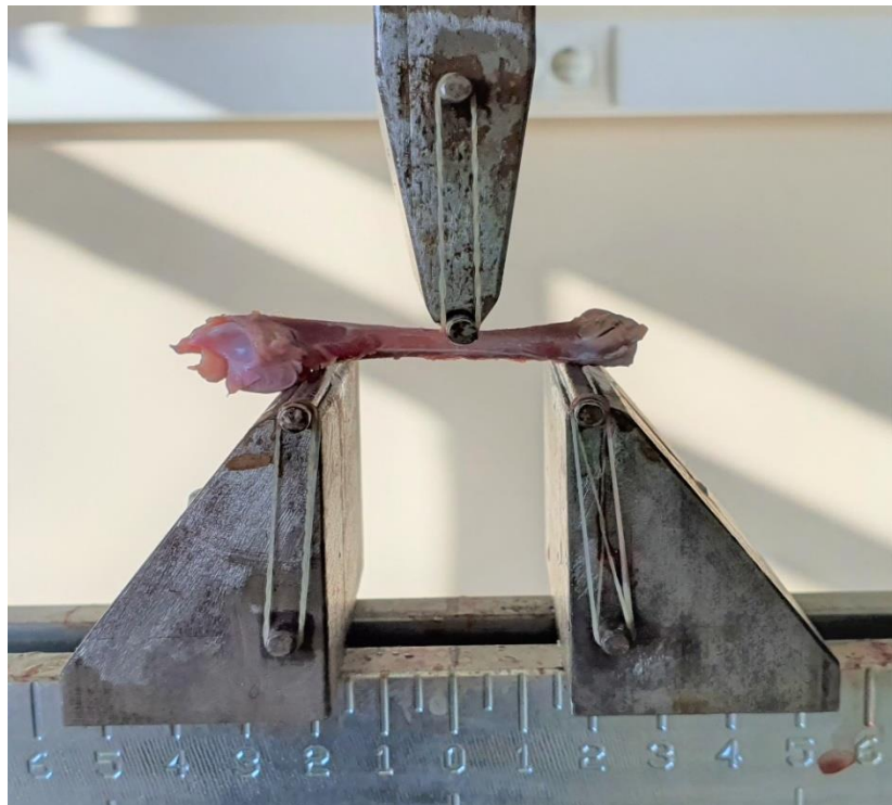
Figure 28. Three-point bending test of ulna.
