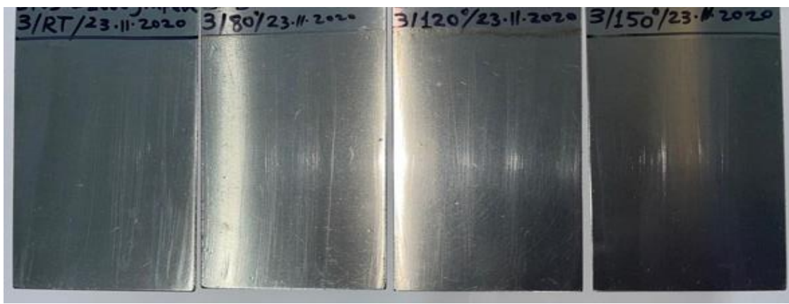
Figure 20. Pictures of ETO-ED900 Coatings (Views of Graphene-Doped Nanocomposite Coatings from Left to Right, at 25°C, 80 °C, 120 °C and 150 °C, Respectively)
