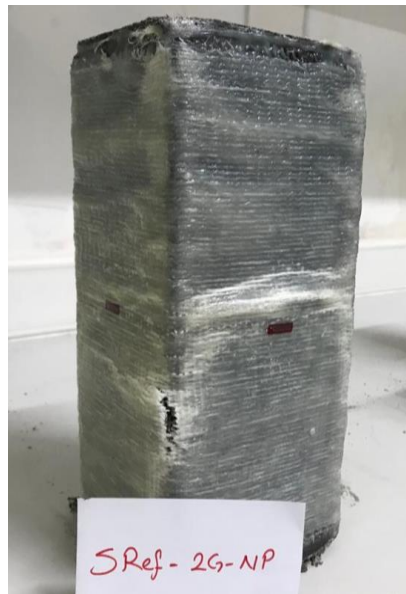
Picture 4.1. The failure mode of specimen, SRef-2G-NP
