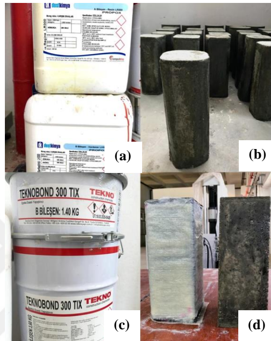
Picture 3.5. (a) The components of primer, (b) specimens after the application of primer, (c) the components of epoxy, (d) the confined and unconfined specimens
