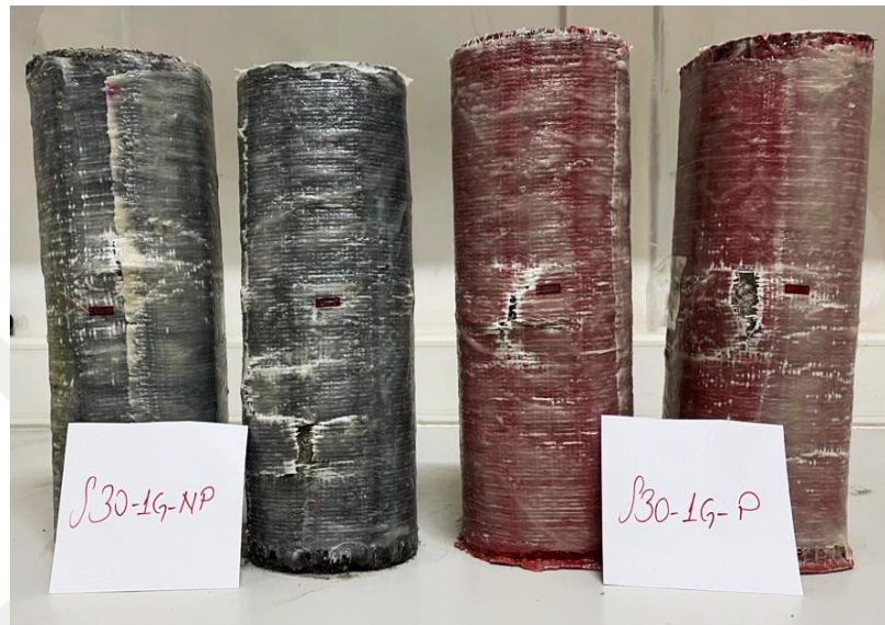
Picture 4.4. Failure modes of S30-1G-NP and S30-1G-P groups
