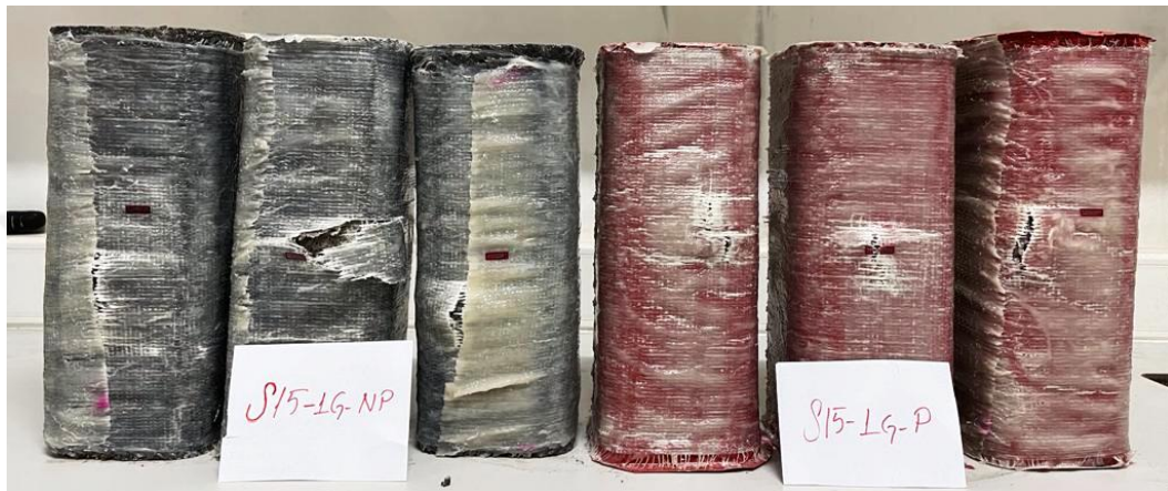
Picture 4.2. Failure modes of S15-1G-NP and S15-1G-P groups
