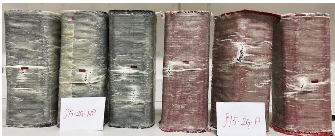
Picture 4.3. Failure modes of S15-2G-NP and S15-2G-P groups
