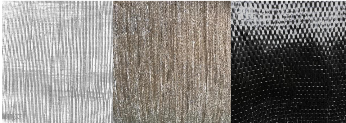
Picture 1.3. Different types of FRP samples; GFRP, FFRP, CFRP
