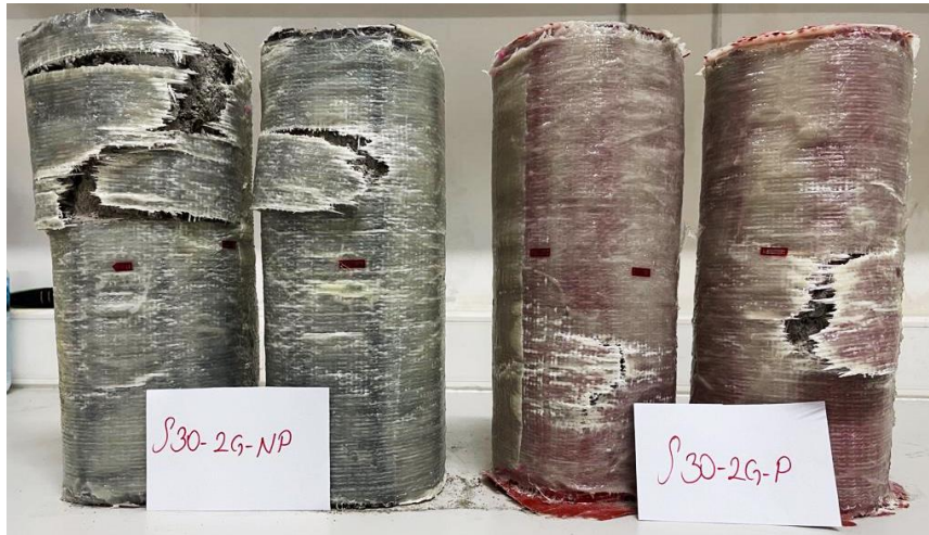
Picture 4.5. Failure modes of S30-2G-NP and S30-2G-P groups
