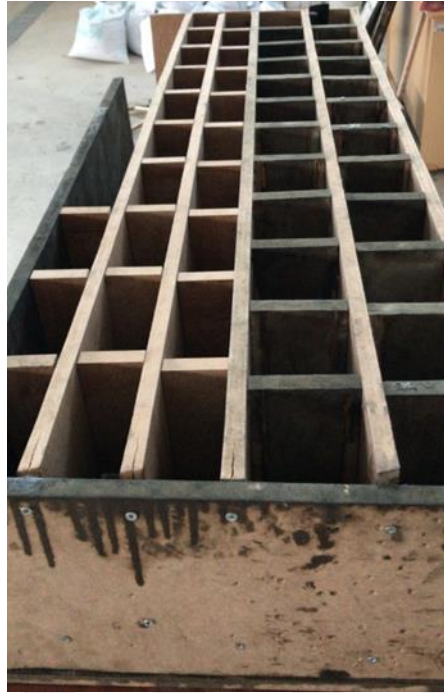
Picture 3.1. The prepared plywood molds
