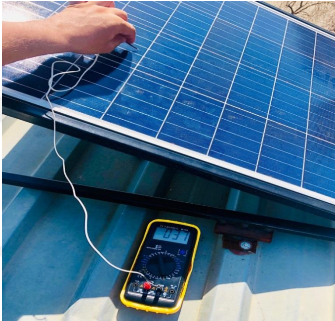
Figure 3.5. K type thermocouple for photovoltaic solar panel surface temperature measurement
