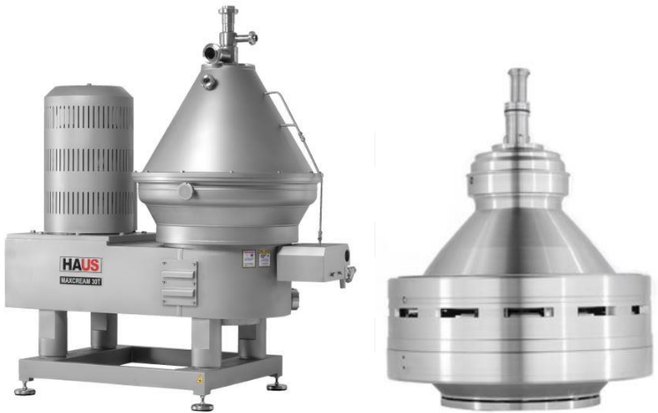
Figure 1.1 Photograph (left) of an ejecting, self-cleaning, disc stack centrifuge. Also shown (right) is a typical disc stack bowl (Courtesy of HAUS Centrifuge Technologies)
