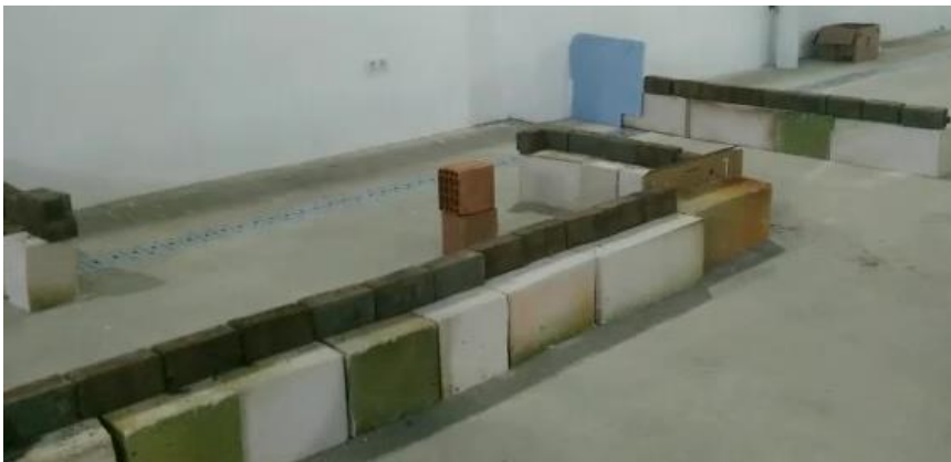
Figure 4.20 Test Bed with Right & Left Corners and Front Right & Left Obstacles (Personal Archive)
