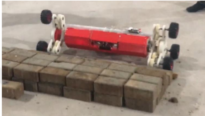
Figure 4.37 Ladder Climbing Test (Personal Archive)
