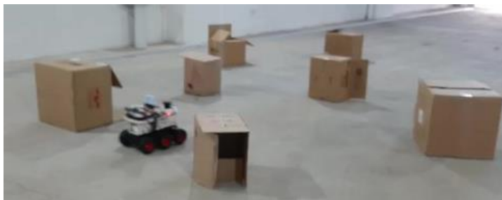
Figure 4.25 Test Bed with Complicated Obstacles (Personal Archive)
