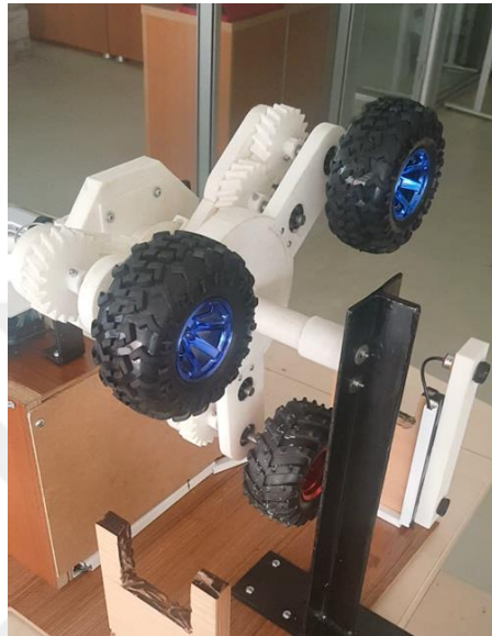
Figure 4.4 Climbing Motion Test (Personal Archive)
