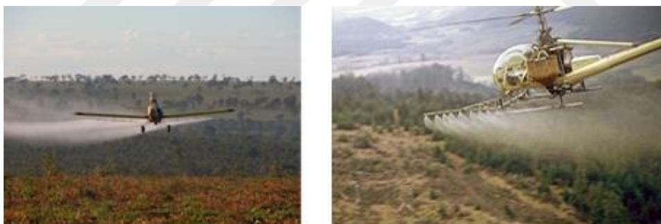
Fig. 2.4. Pesticide drift caused by the distance of the sprayer mechanism of Piloted Aircraft (Beyond Pesticides Daily News Blog, 2019).
