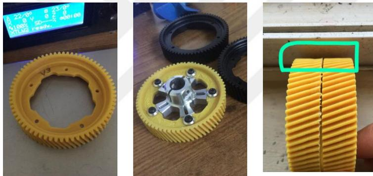
Fig. 4.39. 3D Printed Main Gear.
