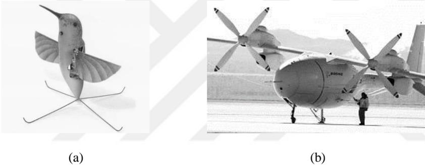
Fig. 2.6. UAVs (a) Hummingbird, (b) Phantom Eye .
