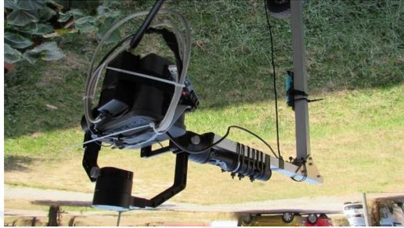
Fig. 4.47. The mounted gimbal and the multispectral camera on the UGV.
