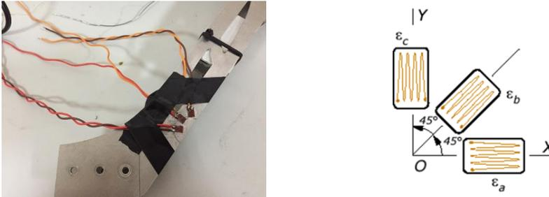
Fig. 3.72. Rosette type strain gauge layout.
