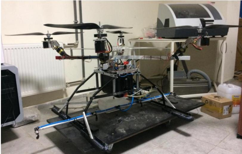
Fig. 4.42. Sprayer UAV.
