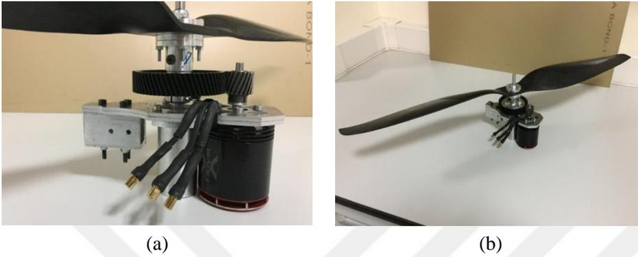
Fig. 3.64. Mounting of the gear reducer and the propeller.
