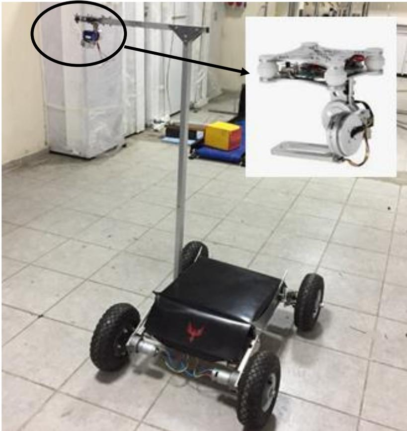
Fig. 3.14. The UGV with the sensor holder.
