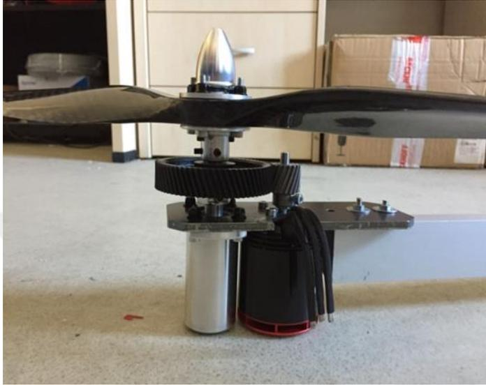
Fig. 4.40. Manufactured gear reducer assemble.
