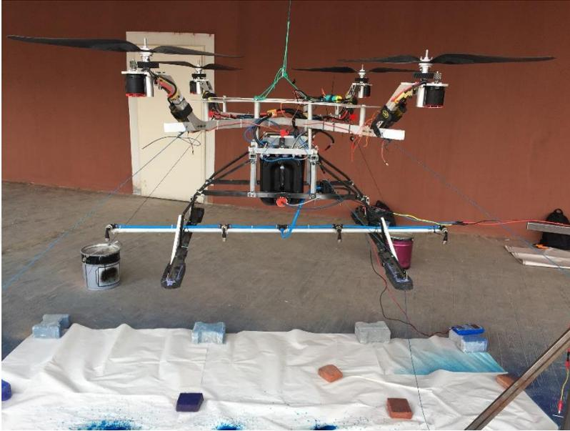
Fig. 4.60. Spraying pattern testing setup.
