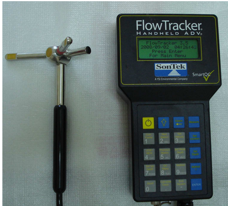
Figure 1. FlowTracker with 2D probe.
