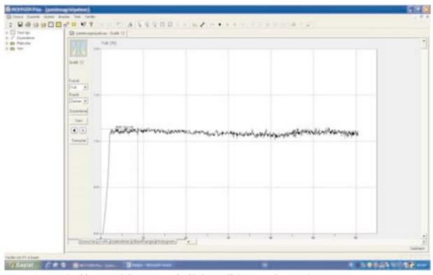
Figure 2. A sample of force-travel distance curve for friction coefficient tests of potato tubers
