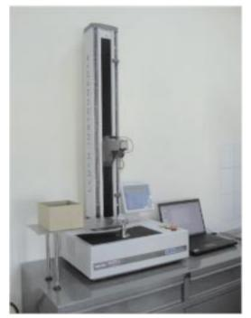
Figure 1. Friction test device
